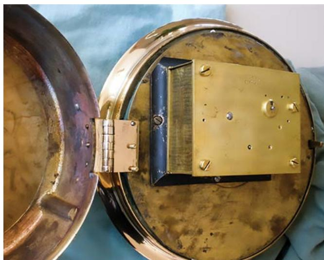
**Figure 14.** The USS *Manhattan* clock and the E. Howard movement with direct dial attachment and dual hinge. PHOTO BY THE AUTHOR.
