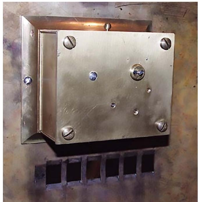
**Figure 20.** The USS *New Ironsides* clock with a Giroud movement attached to the rear of the dial. COURTESY OF JAMES DYSON.
