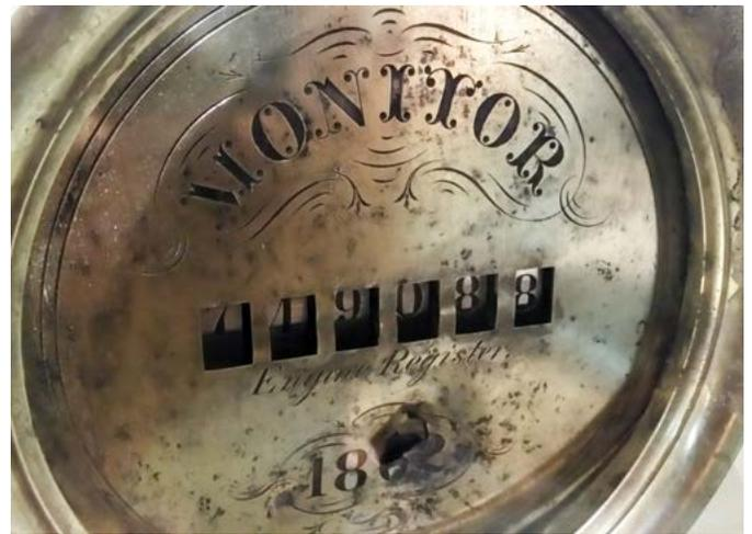
**Figure 17.** The USS Monitor's engine revolution counter. COURTESY OF THE MARINERS' MUSEUM, NEWPORT NEWS, VA.
