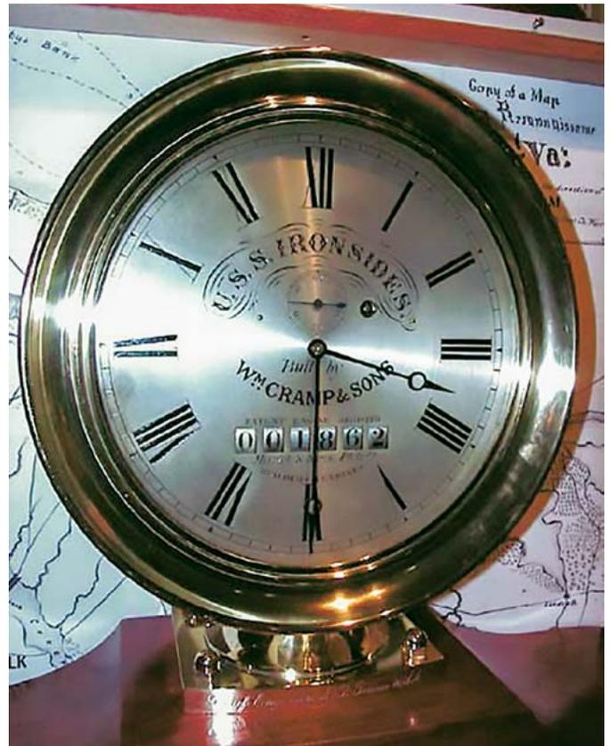
**Figure 18.** Restored USS New Ironsides combination clock and engine revolution counter in a 14" dialed case. The device is on loan from the U.S. Naval Historical Center in Washington, DC, to the Hampton Roads Naval Museum in Norfolk, VA. COURTESY OF JAMES DYSON.
