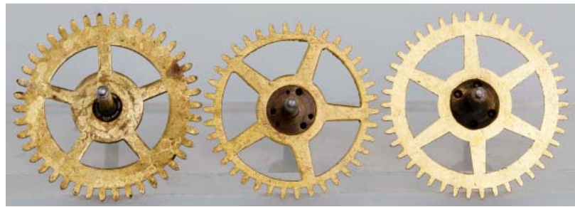
Figure 5I. Three examples of 4th going wheels. Left to right, they are from our featured moment, a "Gordon" model clock movement believed to be 100-percent U.S. as made by New Haven Clock Co., and a movement with a "U.S.A" (No BRITISH MANUFACTURE) New Haven Clock Co. logo within a mahogany mantel clock case with a "British Jerome" logo. See text.
