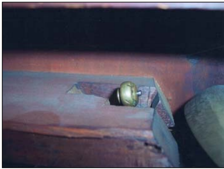
Figure 1P. Bell as seen in Figure 1G with hammer in normal rest position.
