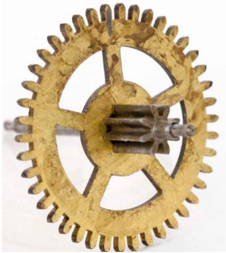
Figure 5G. Front detail of 4th wheel going from movement of Figure 5A, showing solid out pinion and 5-spoked wheel.
