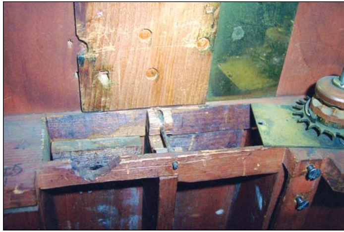
Figure 1H. Clock of Figure 1A with movement removed. Strike cord hooks to bar of center and time cord hooks into hole at right.
