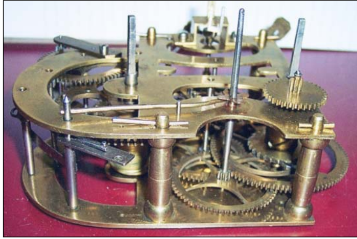
Figure 1M. Strike and time movement of Figure 1G, removed from case, and most of motion work removed, showing important parts of strike and time trains. See text.
