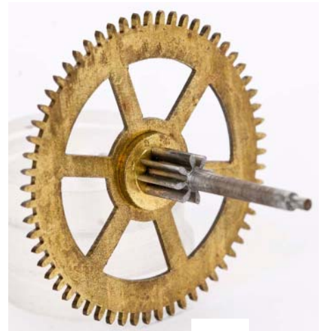
Figure 5F. Rear detail of 2nd wheel going from movement of Figure 5A showing solid cut pinion with wheel collet behind.
