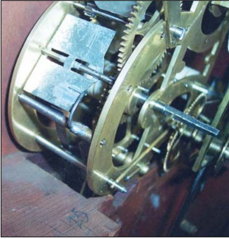
Figure 1L. Top rear view of movement of Figure 1G, showing the ordinary fly and its #4 strike arbor, with a stop pin coming up from the upper strike control arbor.
