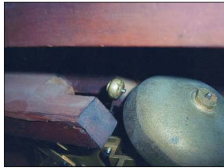
Figure 1Q. Same as Figure 1P with hammer about to hit the bell.
