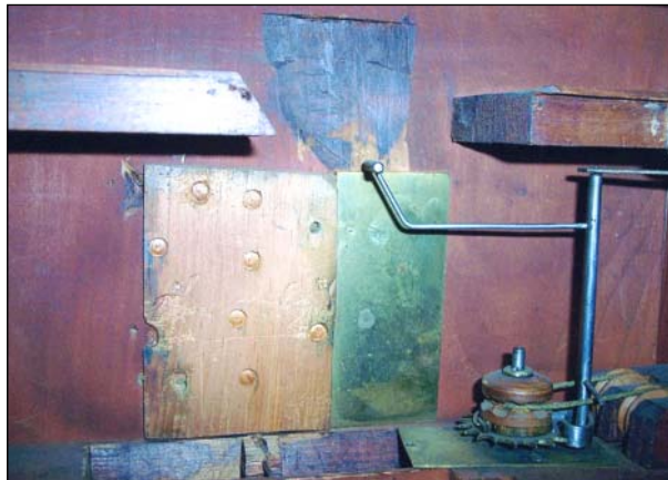
Figure 1J. Clock of Figure 1A, with time-and-strike movement removed, parts of alarm movement remaining. Clock is held in case by two machine screws, which are inserted from the outside of the back, pass through the two holes in the wood spacer, and enter the two holes shown in Figure 1I.
