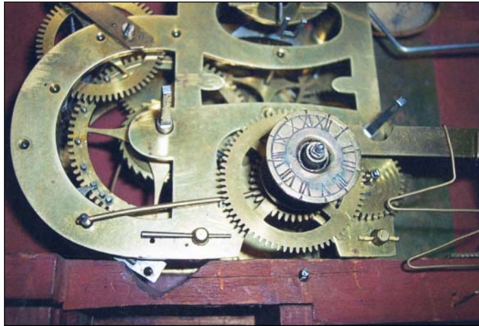
Figure 1N. Lower part of strike and time movement of Figure 1G, removed from case, showing hole at bottom where the strike trip wire attaches. See text.
