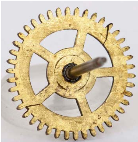
Figure 5H. Rear detail of 4th wheel going from movement of Figure 5A showing wheel riveted directly onto end of its solid pinion. Note 8.2 mm dia. marked ring. See text.
