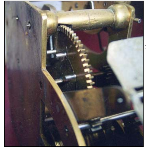
Figure 1K. Detailed view of the upper right square corner in Figure 1I, looking left into movement, showing the strike #2 pin wheel with its pins engaged by the hammer tail. Note the cutaway of the movement post.
