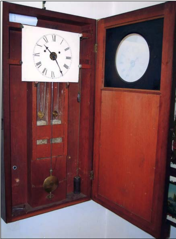
Figure 1D. Door wide open, showing interior of clock of Figure 1A. Note, left to right, strike, time, and alarm cords and weights. Dial repainted some 40 years ago. See text.
