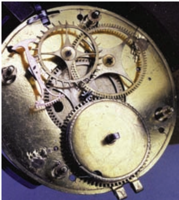
Figure 11, left. The train of the Goddard #282 with the gold rack and going barrel. Figure 12, right. An early Tobias rack lever of approximately the same period.
