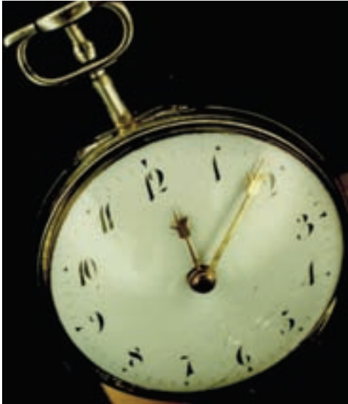
Figure 13, above. A wonderful set of whimsical gold “hands” on Goddard #282 (replacement minute hand made by the author). Figure 14A, below. Goddard rack lever #158 showing steel jeweled balance, lovely pierced eagle cock, and special dished cock screw with blued rim.
