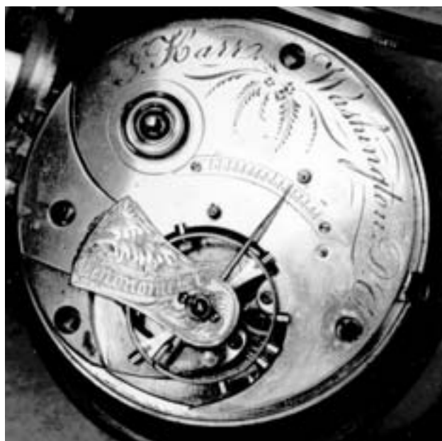
Figure 26, left. A highly experimental pivoted detent escapement by Jacob Karr, Washington. Figure 27, right. Jacob Karr #1.
