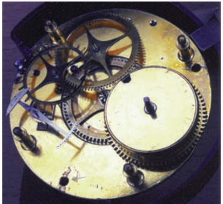
Figure 11, left. The train of the Goddard #282 with the gold rack and going barrel. Figure 12, right. An early Tobias rack lever of approximately the same period.
