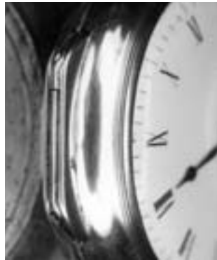
Figures 5A and 5B, right and above. The dial side of Cairns #5, with a very distinctive, but not unique, ringed crystal aperture and a magnificent case of American manufacture. The case is unmarked and has a three-piece hinge. According to David Penney, English case hinges were five pieces exclusively.
