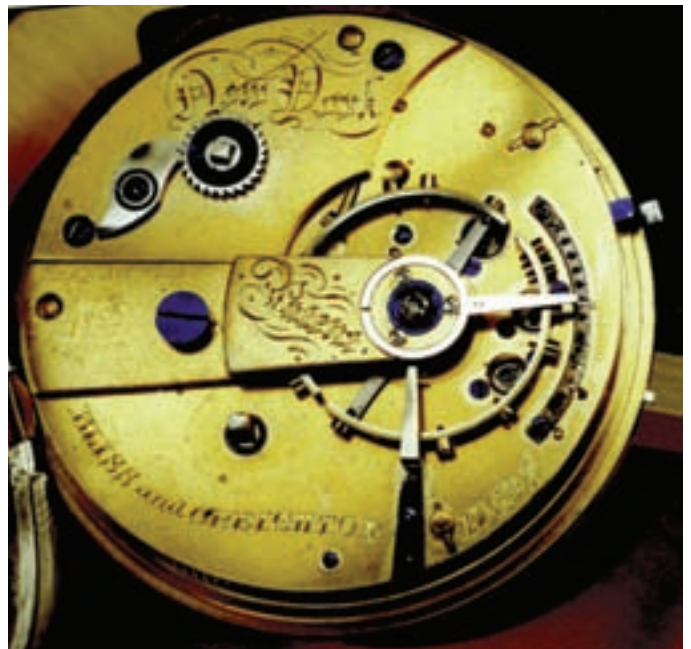
Figure 21, above. Rowley, Shrewsbury (MA?). Engraving was performed after gilding; American watch papers back to the 1840s. This is typical of repairers who purchased finished and gilded watches and added their names. Figure 22, below. Bliss and Creighton, New York, chronometer makers who were more than capable of making any part of this watch, but as far as I can see it is just a very nice contract watch.
