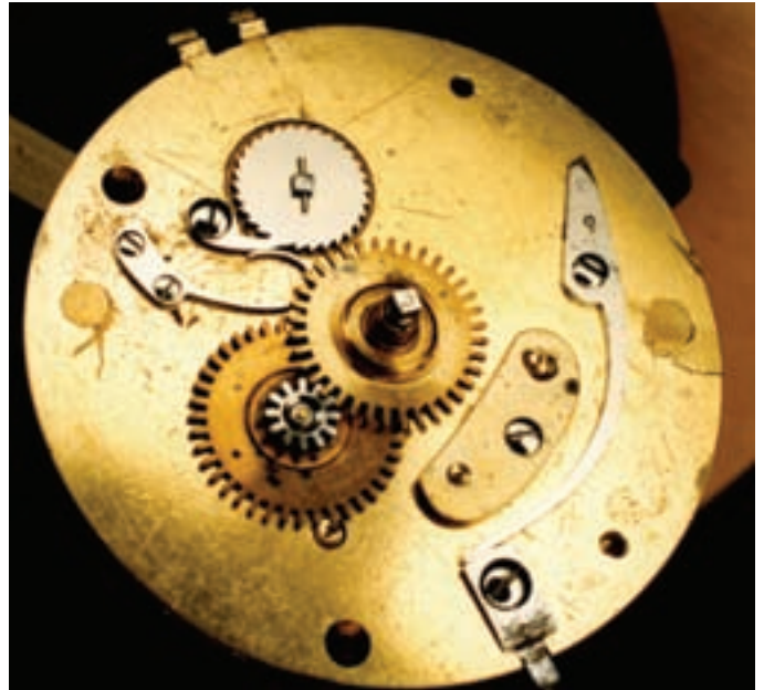
Figure 14D, above. The pillar plate of Goddard #158 after restoration.
