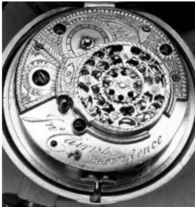
Figure 1. John Cairns #5, notice the mixing of upper and lower case letters in Providence, the roughly pierced and engraved cock, definitely not of London manufacturing quality. Also notice that there is really almost no decorative engraving except for the rather whimsical indicator hand. This watch is featured on the front cover.
