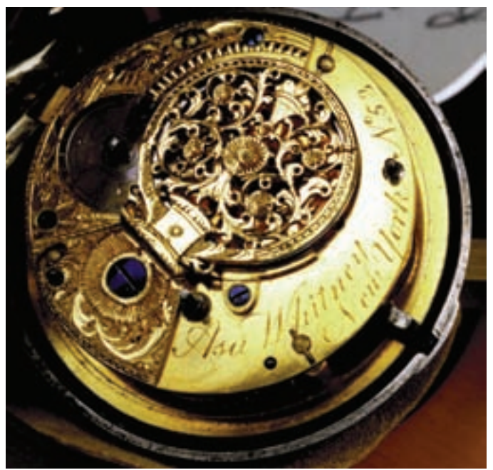
Figure 17, left. Dial side of Fatton #9; notice the ungilded bridges and wheels. Figure 18, right. By my definition this is an American watch; Asa Whitney, #53, Whitney's number, New York. Notice that the reliefs in the regulator and cock foot have been elongated so that the entire top plate could be removed to adjust the escapement without removing the balance or those two plates. Basically, he at least finished the watch, bringing it to time.
