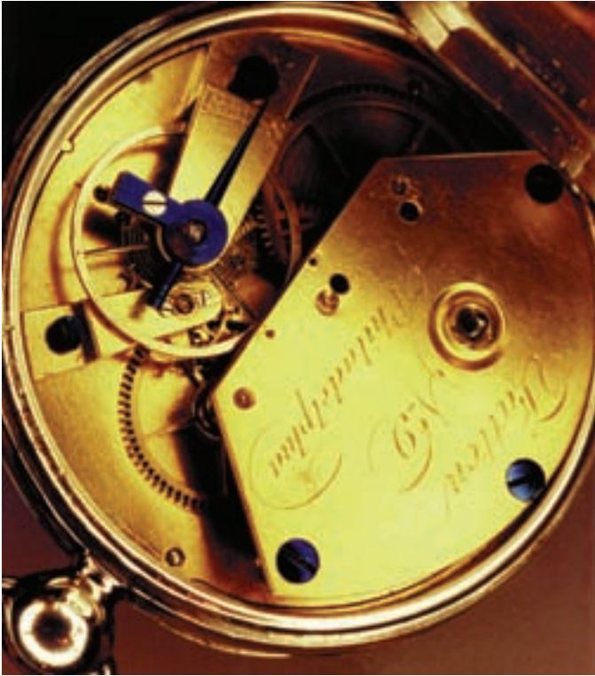
Figure 15, left. Fatton #9, eleve de Breguet, Philadelphia 1832-9. The only known Breguet style ruby cylinder made in the U.S. This watch has a gold balance, a symmetrical train, ungilded wheels, and an English case. The replacement cylinder carriage was made by the author. The English case indicates that the watch was most likely started in England prior to Fatton's arrival in the U.S. Figure 16, right. Dial side of Fatton #9 showing the single screw holding on dial regulator style layout. The matching key was a wonderfully lucky find at a NAWCC National Convention. All hands have been replaced by the author. The bulls-eye crystal creates the refracted second hand.
