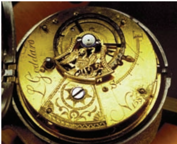
Figure 13, above. A wonderful set of whimsical gold “hands” on Goddard #282 (replacement minute hand made by the author). Figure 14A, below. Goddard rack lever #158 showing steel jeweled balance, lovely pierced eagle cock, and special dished cock screw with blued rim.
