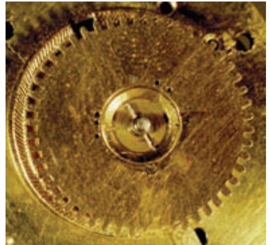
Figure 9, left, Cairns #5, and Figure 10, right, Goddard #282, showing the fusee wheels secured to the fusee without any washer, just with the taper pin alone as the washer and retainer.
