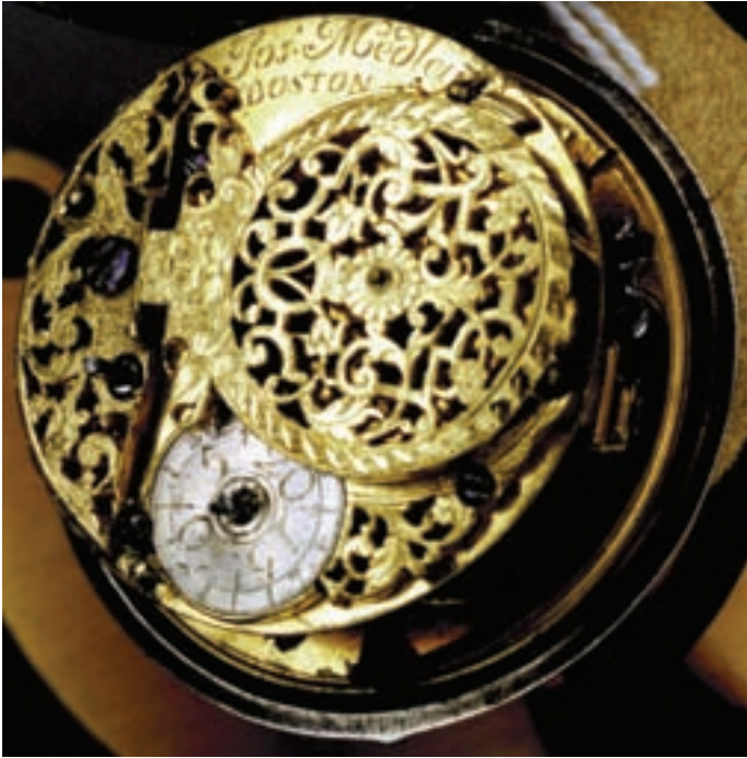
Figure 20, above. Josia Medley, Boston, ca. 1732. I believe this to be the earliest known documented American contract watch, most certainly of London manufacture, with broad footed cock and Egyptian columns.
