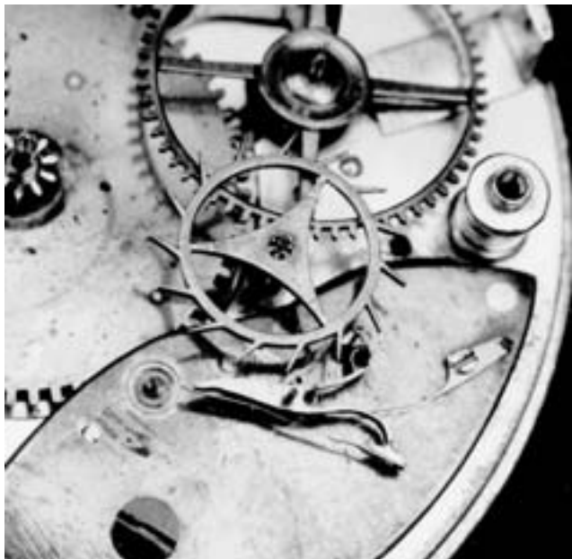
Figure 26, left. A highly experimental pivoted detent escapement by Jacob Karr, Washington. Figure 27, right. Jacob Karr #1.
