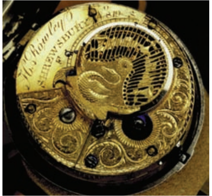
Figure 21, above. Rowley, Shrewsbury (MA?). Engraving was performed after gilding; American watch papers back to the 1840s. This is typical of repairers who purchased finished and gilded watches and added their names. Figure 22, below. Bliss and Creighton, New York, chronometer makers who were more than capable of making any part of this watch, but as far as I can see it is just a very nice contract watch.
