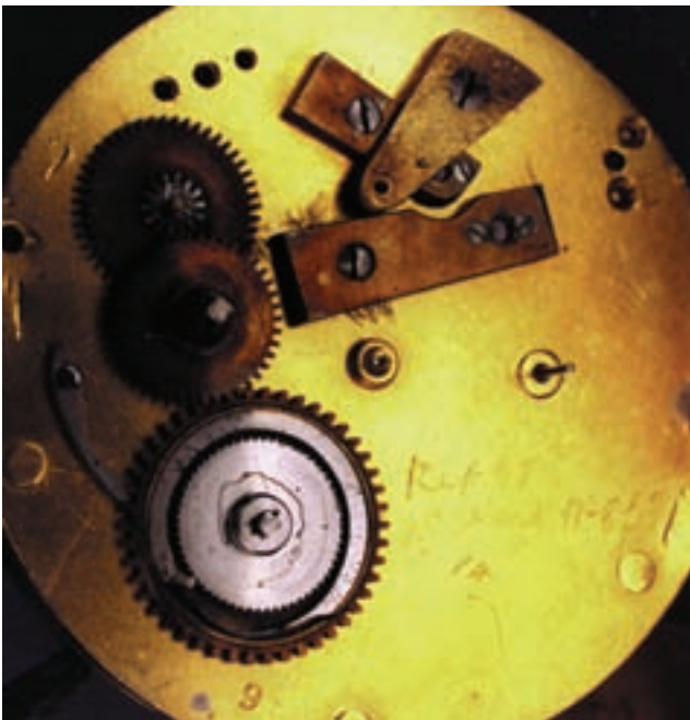
Figure 17, left. Dial side of Fatton #9; notice the ungilded bridges and wheels. Figure 18, right. By my definition this is an American watch; Asa Whitney, #53, Whitney's number, New York. Notice that the reliefs in the regulator and cock foot have been elongated so that the entire top plate could be removed to adjust the escapement without removing the balance or those two plates. Basically, he at least finished the watch, bringing it to time.
