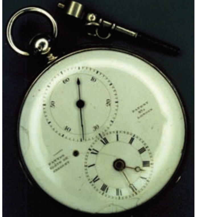
Figure 15, left. Fatton #9, eleve de Breguet, Philadelphia 1832-9. The only known Breguet style ruby cylinder made in the U.S. This watch has a gold balance, a symmetrical train, ungilded wheels, and an English case. The replacement cylinder carriage was made by the author. The English case indicates that the watch was most likely started in England prior to Fatton's arrival in the U.S. Figure 16, right. Dial side of Fatton #9 showing the single screw holding on dial regulator style layout. The matching key was a wonderfully lucky find at a NAWCC National Convention. All hands have been replaced by the author. The bulls-eye crystal creates the refracted second hand.
